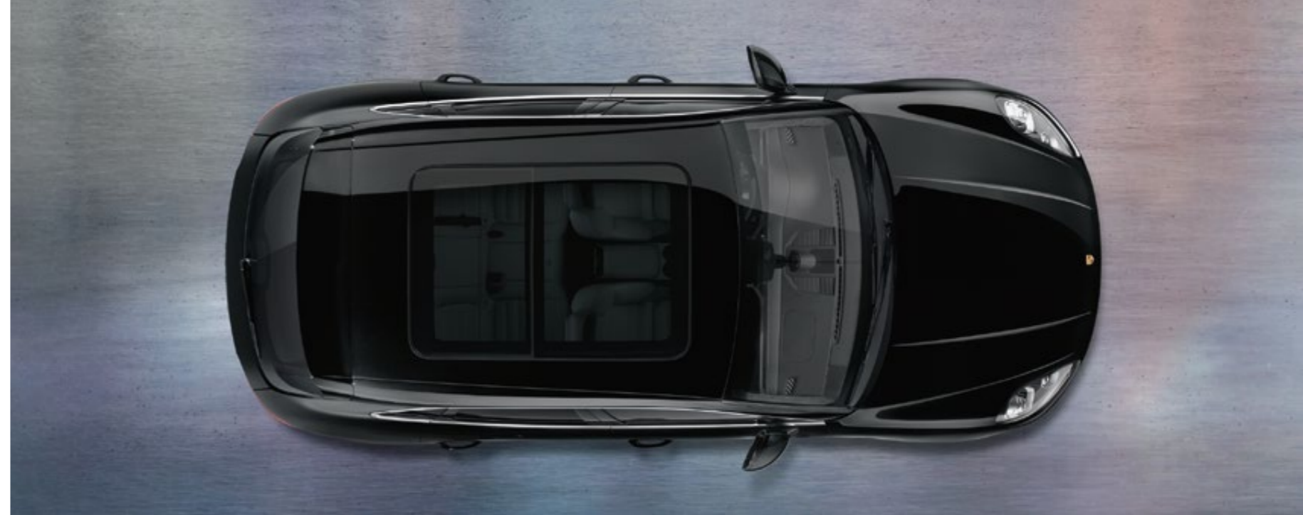
Panoramic roof system
