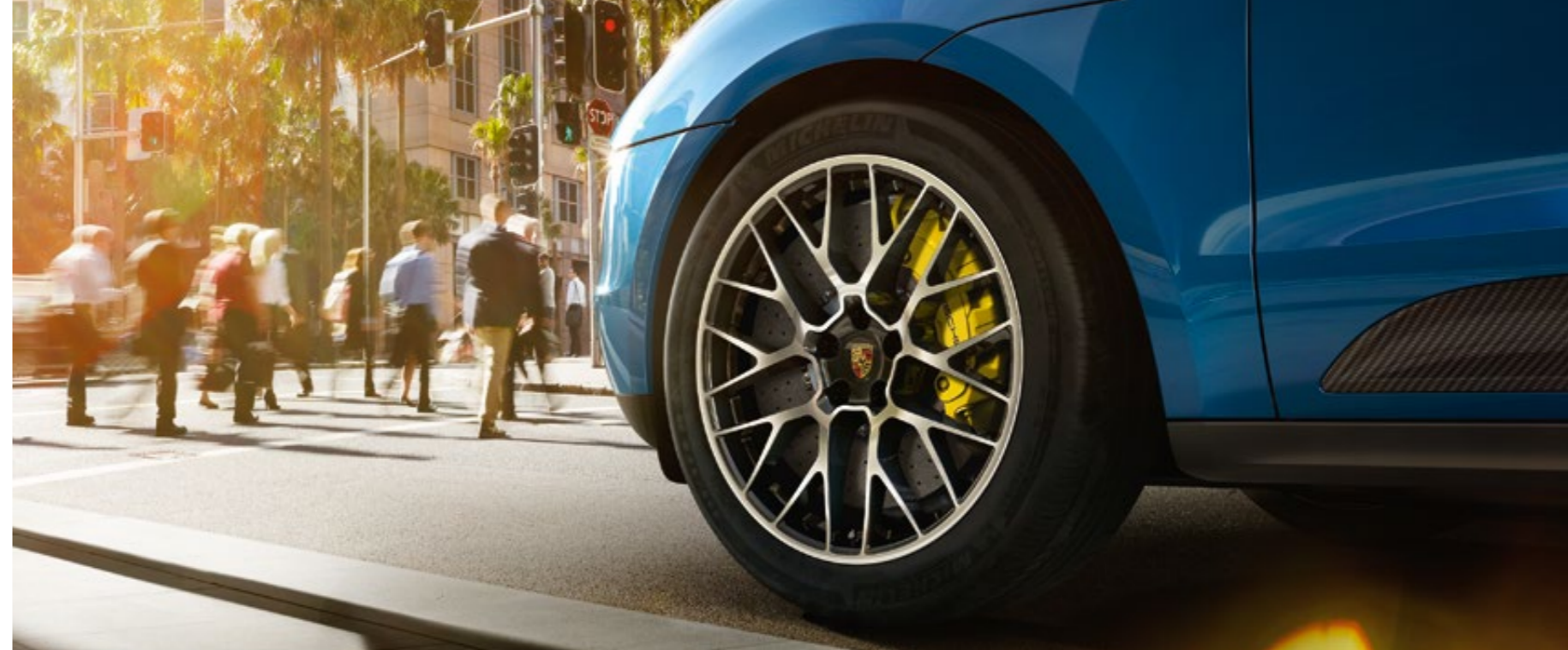
Porsche Ceramic Composite Brake (PCCB) on the Macan S
