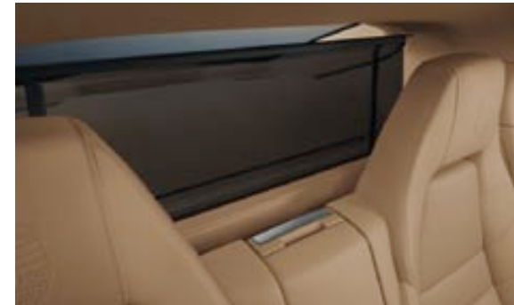
Fixed luggage compartment cover with electric roll-up sunblind for behind the rear compartment
