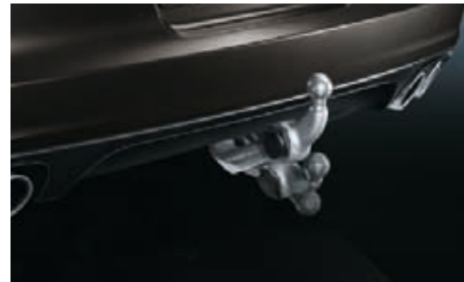
Electrically extending towbar system
