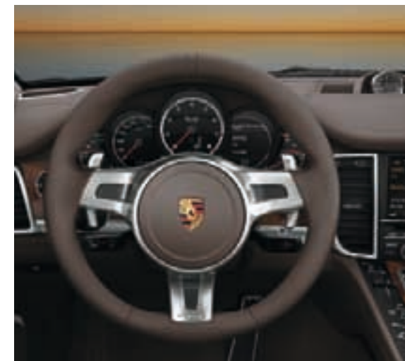
Three-spoke sports steering wheel with gearshift paddles
