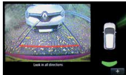
Reverse parking camera system Front and rear parking sensors with reverse parking camera, which displays the image on the navigation system screen alongside guidance aids.
