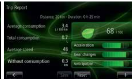
Vehicle information The fun 'Eco Driving' coach gives you handy tips to improve your driving style and reduce your fuel consumption.
