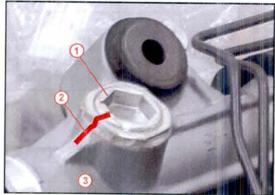
1 Rack Guide Spring Cap 2 Matchmark 3 Gear Box Housing
