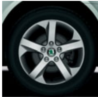
Proxima 6.5J x 16" alloy wheels with 205/55 R16 tyres are standard on the 118TSI and 103TDI models.
