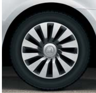
6.5J x 16" steel wheels for 205/55 R16 tyres with Tecton hub covers
