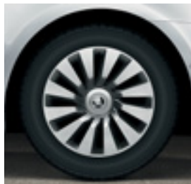
6.5J x 16" steel wheels for 205/55 R16 tyres with Tecton hub covers
