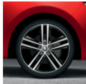
7.0J x 17" Ray alloy wheels for 215/40 R17 tyres, in black design exclusive to the Style Pack.
