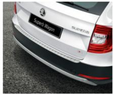
Enhancing its outdoor use a **protective** silver strip on the loading edge of the boot prevents damage when loading or unloading objects.
