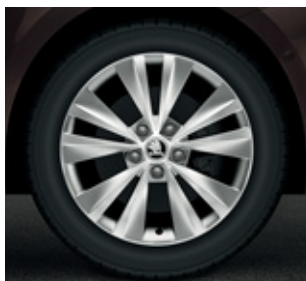
7.5J x 17" Twister alloy wheels for 225/45 R17 tyres.
