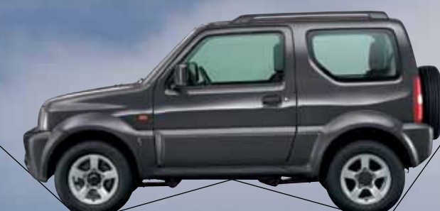
A 34° Approach angle B 31° Ramp breakover angle C 45° Departure angle (default setting, unloaded Jimny Sierra)
