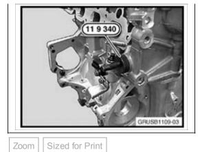
10. Fit the chain tensioner (Special Tool 11 9 340) without the seal ring and with the lock nut loose. Pretension the chain tensioner with Special Tool 00 9 250 to 0.6 Nm. Finger-tighten the lock nut on Special Tool 11 9 340.
