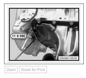
8. Install the locating pin (Special Tool 11 9 590) to lock the position of the engine.
