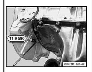
5. Install the locating pin (Special Tool 11 9 590) to lock the position of the engine.
