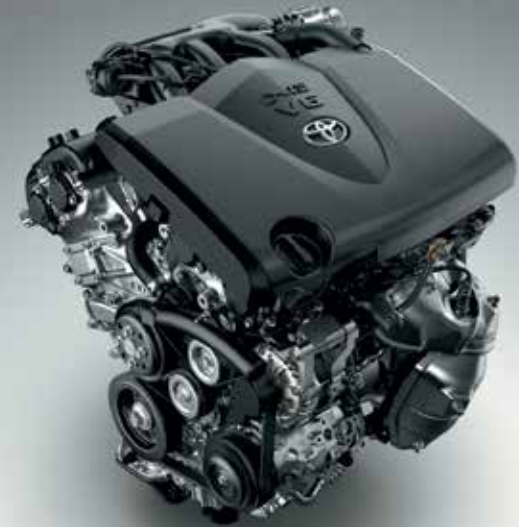
3.5L Dual VVT-iW V6 petrol engine
