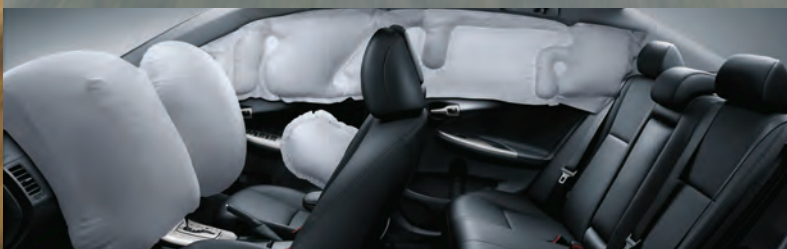
Driver and front passenger SRS airbags, front seat side airbags, full length side curtain shield airbags and driver's knee airbag. Ultima model shown.
