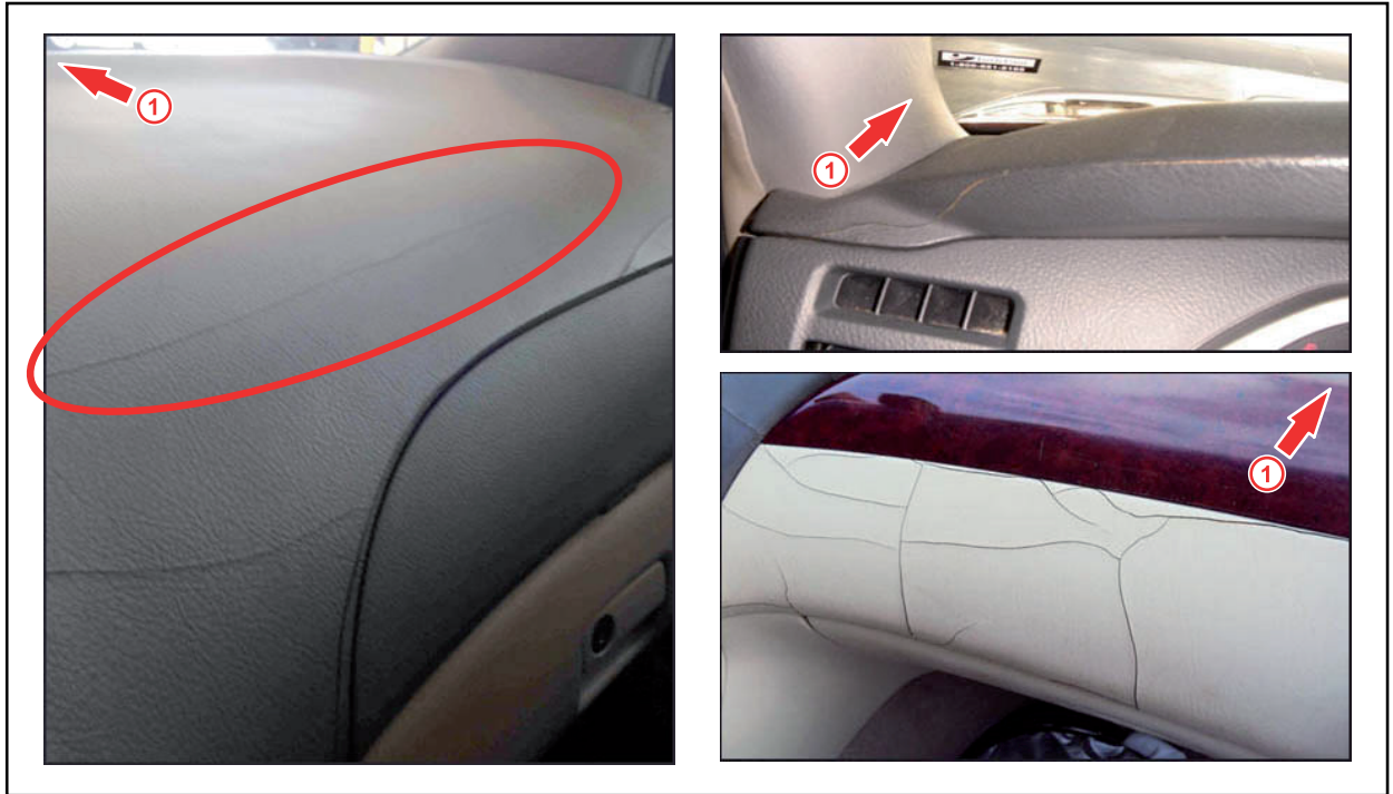
Figure 3. Examples of Cracked Condition
