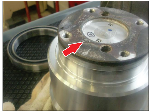
Figure 7. Excessive Rust/Corrosion Buildup on Top of Coupling Body
