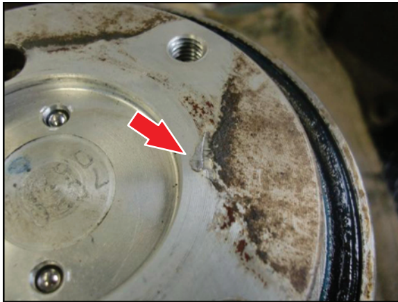
Figure 6. Damage Where Propeller Shaft Contacts Coupling Body
