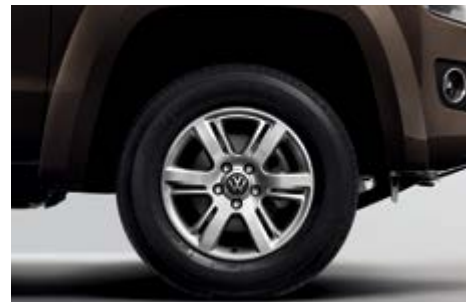
17-inch "Aldo" alloy wheels, including flared wheelhouses. With 245/65 R17 111T tyres.
