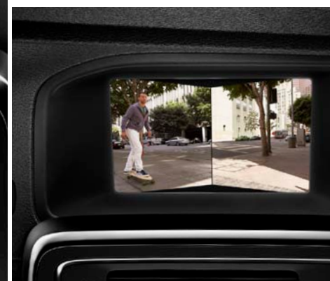
▶ Front blind view camera
