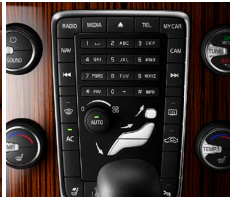
Electronic Climate Control (ECC)
