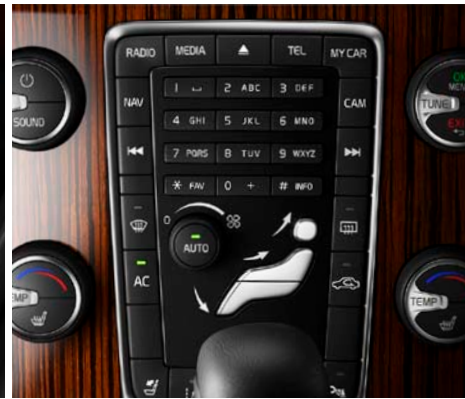
Electronic Climate Control (ECC)
