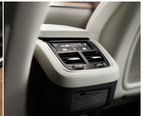
The four-zone climate system can be controlled from the centre display touchscreen, or a graceful touch control panel at the end of the tunnel console.
