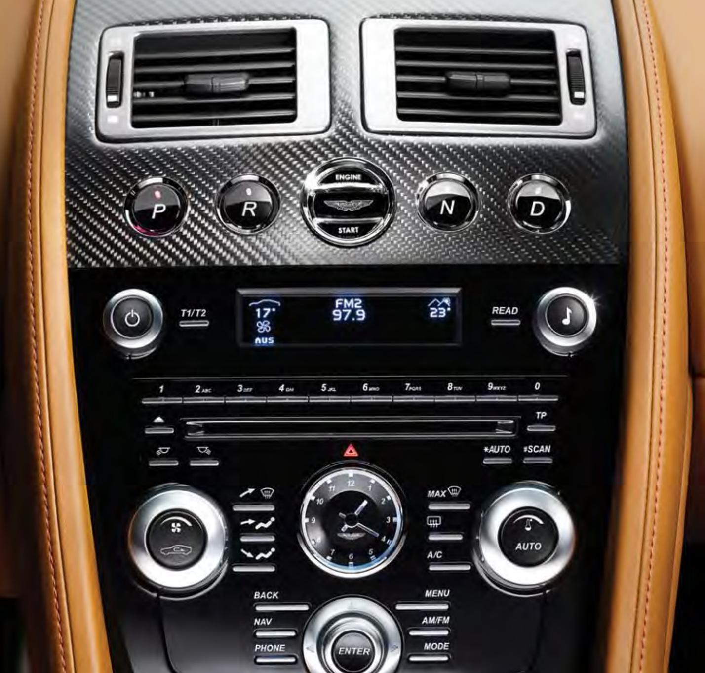
Distinguishing the Carbon Edition is the carbon-fibre facia with a carbon weave that has been precisely positioned to follow the form of the dashboard. Only by hand can the fibres be laid to create a perfectly aligned weave.
