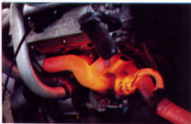
Biturbo engine on the dynamometer during extremely heavy endurance tests at maximum power and speed
