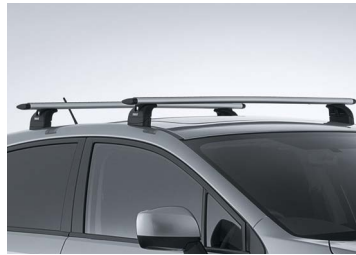
ROOF CROSS BARS
